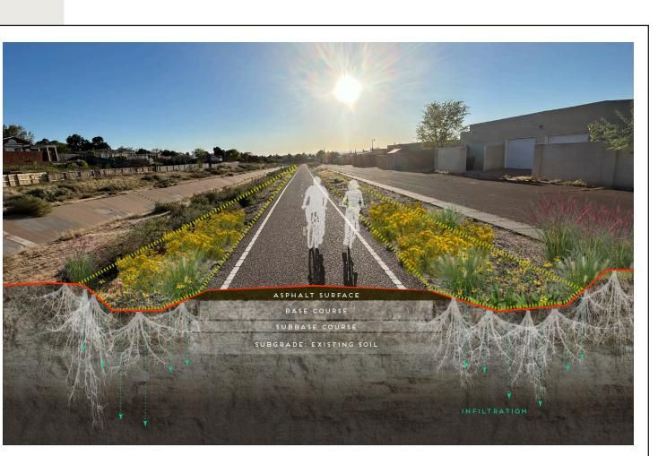
Stormwater management using green infrastructure practices involves keeping and using water close to its point of origin. To help filter and capture stormwater runoff without losing it directly to the arroyo channel, this project proposes adding gently sloping depressions on either side of the biking/walking path, planted with dense native vegetation and grasses. Bioswales such as these filter stormwater runoff as it flows through the swale, allowing it to slowly infiltrate into the ground.
